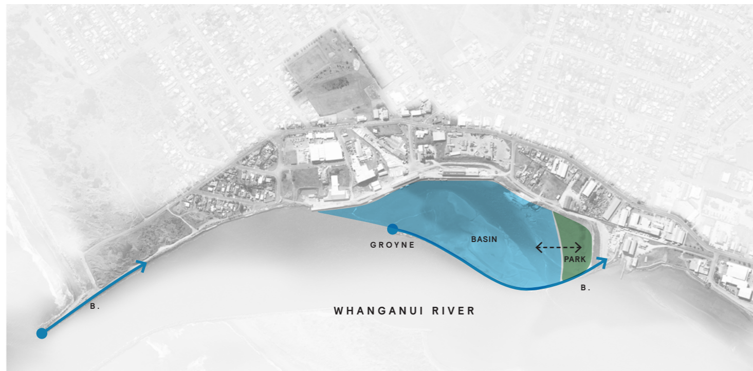
003 REINSTATE THE PORT BASIN Recreating the Port Basin unlocks the working and recreational potential of the port. This is achieved by: A. Dredging the basin to enable deep water access adjacent the wharf edges and a fully wet basin at all tides for recreational activity. B. Reinstating river training wall to separate the basin from the River. C. Use the material from the dredging to reclaim new public park that supports recreational activity. D. Reinstating North Mole as an important regional destination and landmark for the port.
